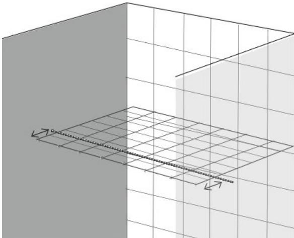
Figure 3: Support wire position
