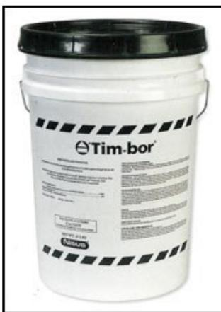
A preservative that is highly toxic to wood-destroying insects and fungi, as well as preventing infestation when properly applied; yet treated wood is non-toxic to humans or animals. Tip: One 6-gal. pail of powdered concentrate makes up 27 gal. of mixed product, or enough to cover 1950 sq. ft. This is enough to coat the exterior of a log house about 30 ft. x 50 ft. with 9-1/2 ft. sidewalls.
